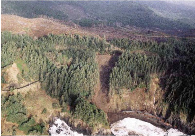
Highway 101. ODOT has identified 4,000 culverts under the entire length of Highway 101.” Culverts are significant because as they age they become less functional. During rainstorms, if culverts can’t pass water, the water backs up behind the road bend making the hillside highly vulnerable to catastrophic failure. A leading cause of the Cape Foulweather slide was inadequate drainage under Highway 101 (combined with unstable geology and outdated building practices employed many years ago).
